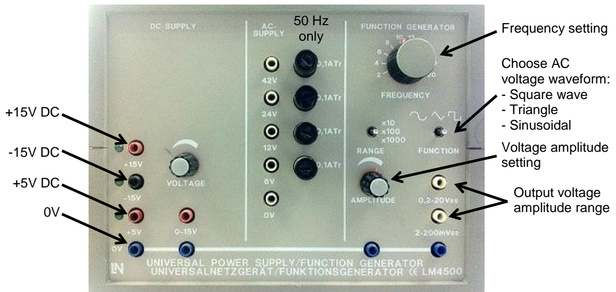
Figure 8: Universal power supply (LM4500)
